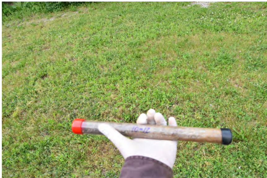
Typical soil sample recovered from boring GP-1. Sample consists of coarse sand with trace of gravel and clay.
