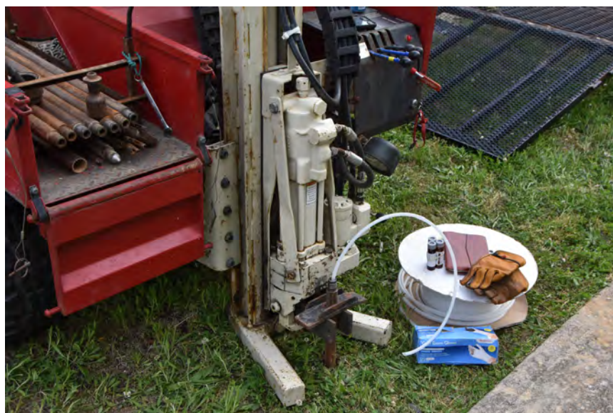
Recovering a ground water sample from temporary well GP-1.
