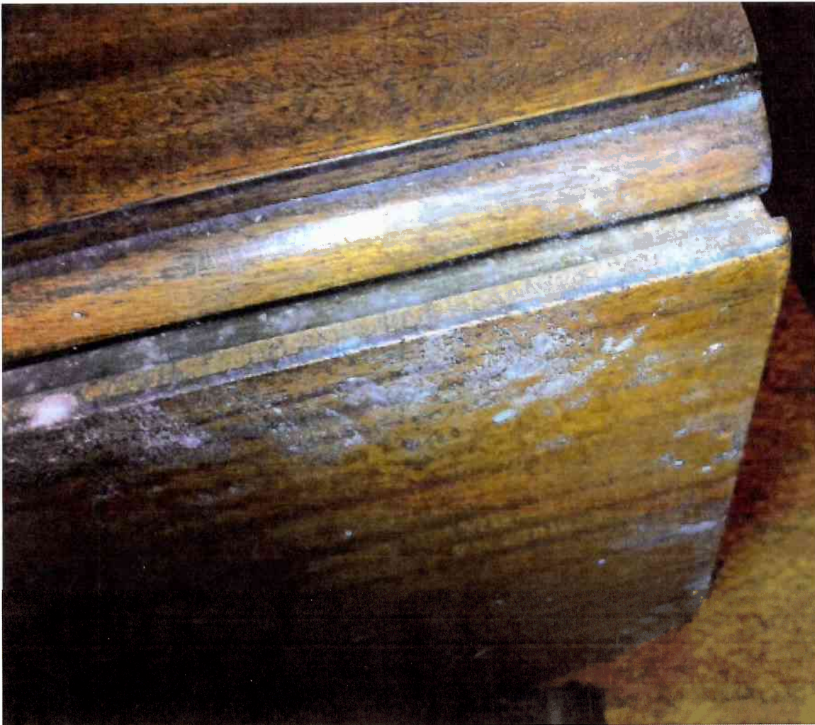
Fungal growth on basement contents.
